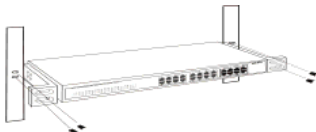
Figure 2. Mount the Switch in the rack
